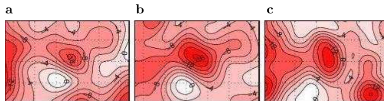
Figure 3: Subsidence estimation (mm) using (a) leveling, (b) PS-InSAR and (c) PS-InSAR with a higher spatial density. PS-InSAR data has been processed by TRE/NPA for NAM. There is a constant bias in each estimation due to the differential character of the observations.
