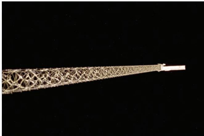
View from the Commander’s seat of the SRTM mast and outboard antennas 60 meters away.
