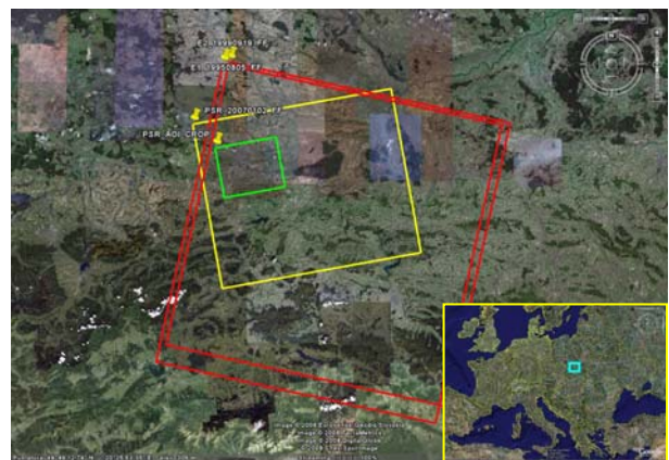
Figure 1. Yellow frame refers to the ALOS PALSAR acquisition (PRS_70070102), green frame encloses the AOI, red frames refer to ERS acquisitions E1_19950805 and E2_19990919. Inset shows the location of the study area.
