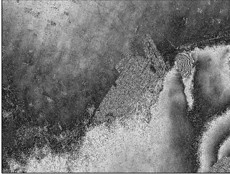
Figure 26: Topographic interferogram of the Cerro Prieto area. Perpendicular baseline B_{\perp} = 310 meters, height ambiguity z_{2\pi} = 30 meters.
