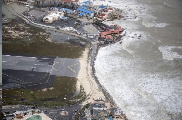
Figure 21: Maho Beach completely washed away and moved up the beginning of the runway (NRC, 2017)
