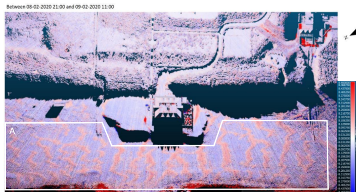
Figure 2.3: The height differences of the beach between 8-2-2020 21:00 and 9-2-2020 11:00 (adapted from Schreijer, 2021). Red indicates an increase in height, blue indicates a decrease in height. Sand waves are clearly visible in area A.
