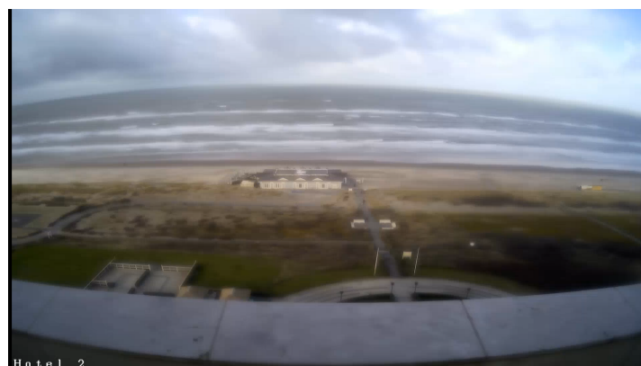
Figure 4.4: The image quality on March 10, 2020 is reduced by rain. This rain disturbed the point cloud of that day.
