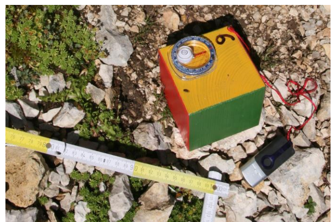
Figure 29. Cube with GPS, compass and level for model orientation.
