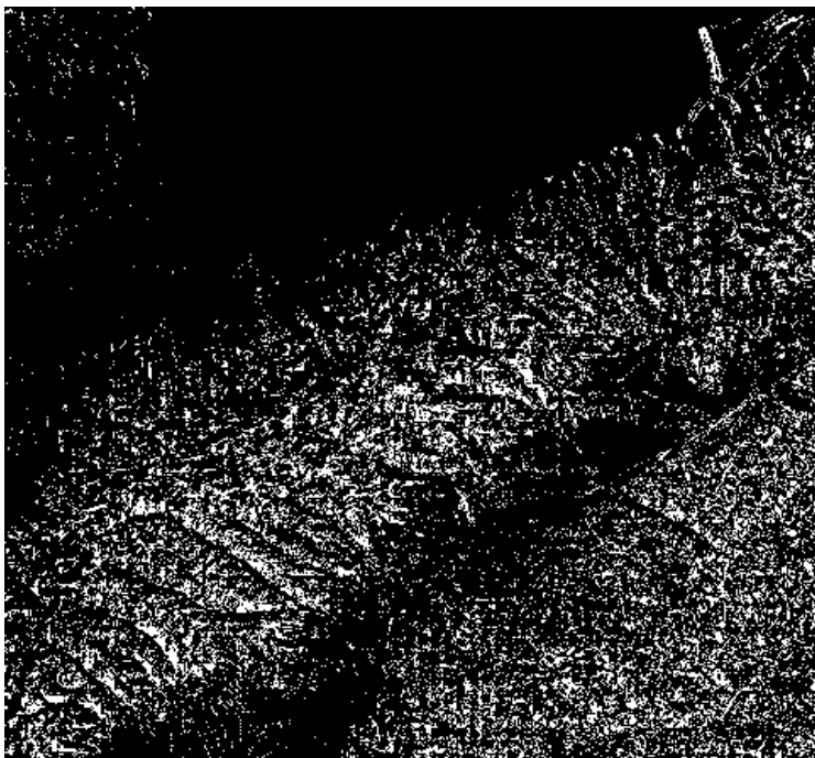
Figure 37: Difference plot between ASTER GDEM and SRTM, white color is for a difference >30 or <-30 meters
