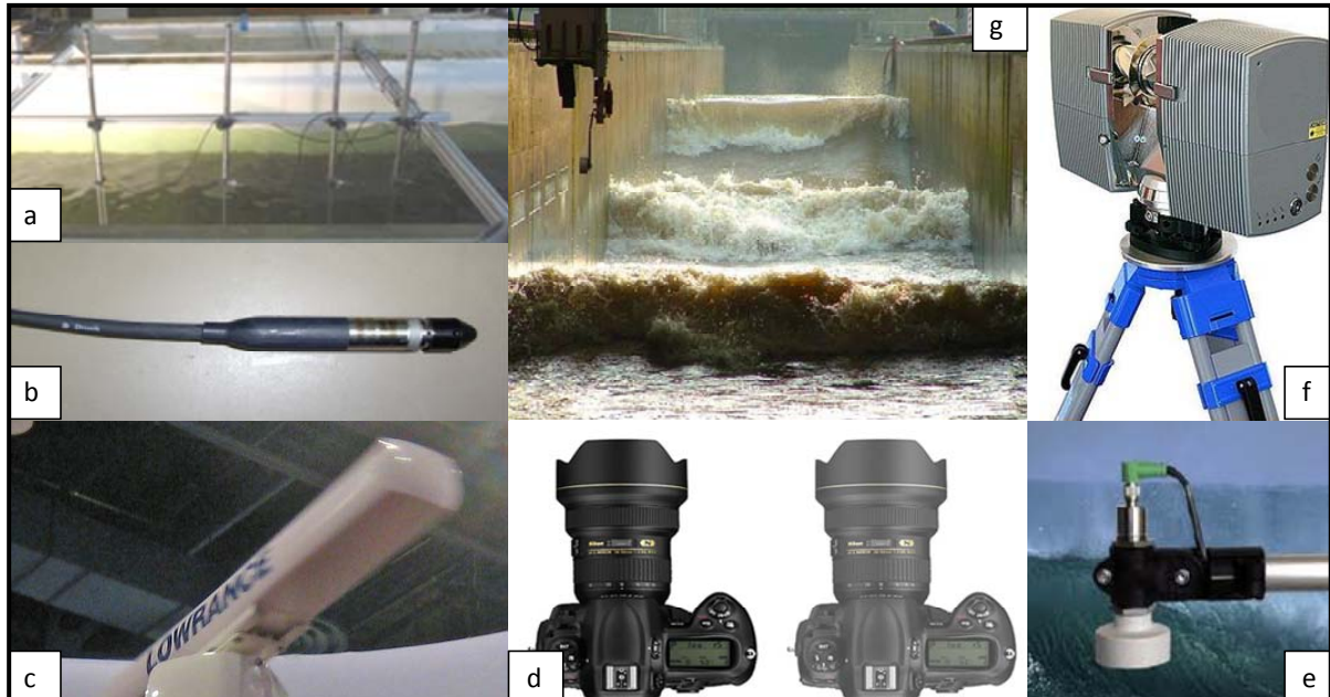
Fig. 7: Water surface measurement devices. a: wave probes (LWI Braunschweig), b: pressure meter ( www.fs.fed.us ), c: RADAR ( www.panbo.com ), d: stereo image photogrammetry ( www.qwerty.com ), e: ultrasonic altimeter ( www.act-us.info ), f: LIDAR ( www.translationdirectory.com ), g: waves in hydraulic measurement (Deltaflume, Deltares)
