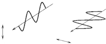
Figure 7: Principle of polarization; Left: horizontal polarization, Right: Vertical polarization [7]
