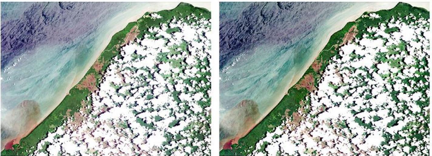
Figure 4: Left: Level 1C Input, Bands 2-4; right: Level 2A Output, Bands 2-4, RGB composite images
