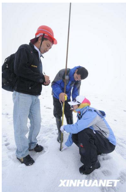
Figure 3-1 An example of a field measurement with marker poles on 4800 m by the CAREERI researchers on Yulong Snow Mountain (XINHUANET)
