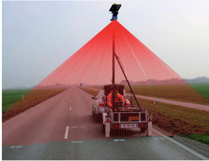
Figure 2.4: The Pavescan system with a schematic laser bundle. (Illustration from [Mennink, 2008])
