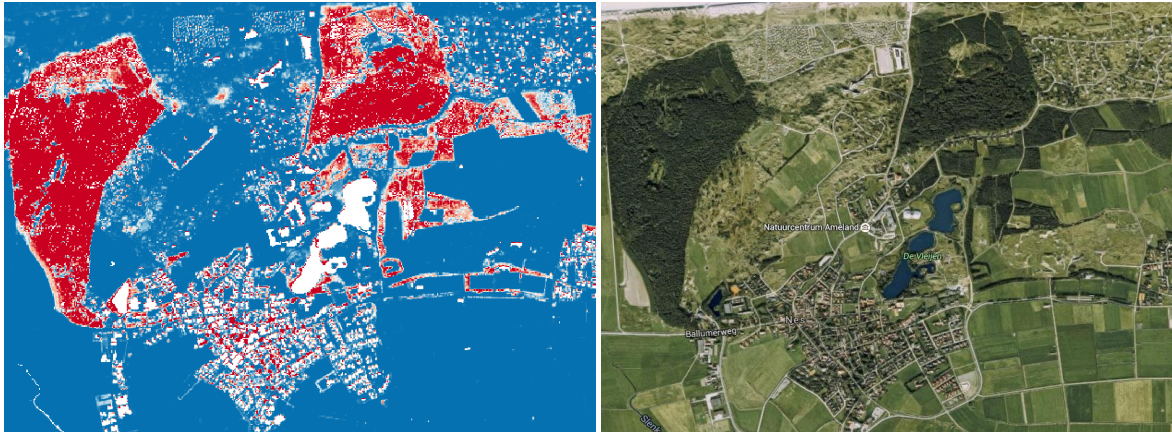
Figure 19 Left: difference between raw and filtered data in AHN. Right: image taken from Google Maps of the same area. The area is the village of Nes on Ameland.
