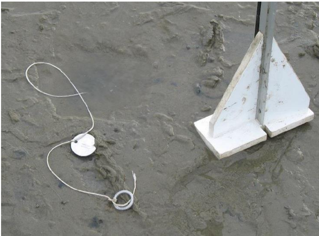
Figure 4 String used to measure sedimentation speed in the research of Johan Krol [7]
