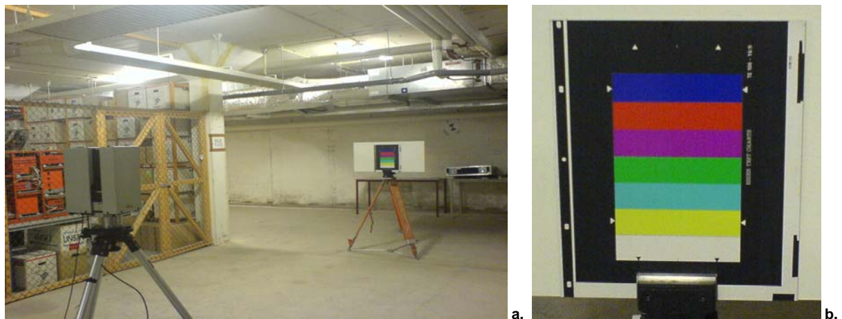
Figure 6.2: a. The colour experiment set-up with left the Leica HDS4500 scanner and right in the picture the tripod with the white plate and the colourChart placed in front, b. a close up of the colourChart in the angle m. device (photos: Van Ree, 29-03-2006).
