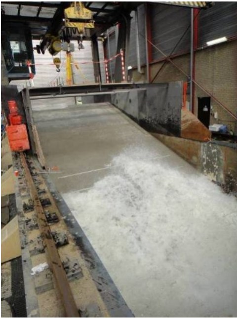
Figure 6. TLS measurement of breaking-wave profiles on a slope. Left: setup. Right: example of result (every line represents a different time step).
