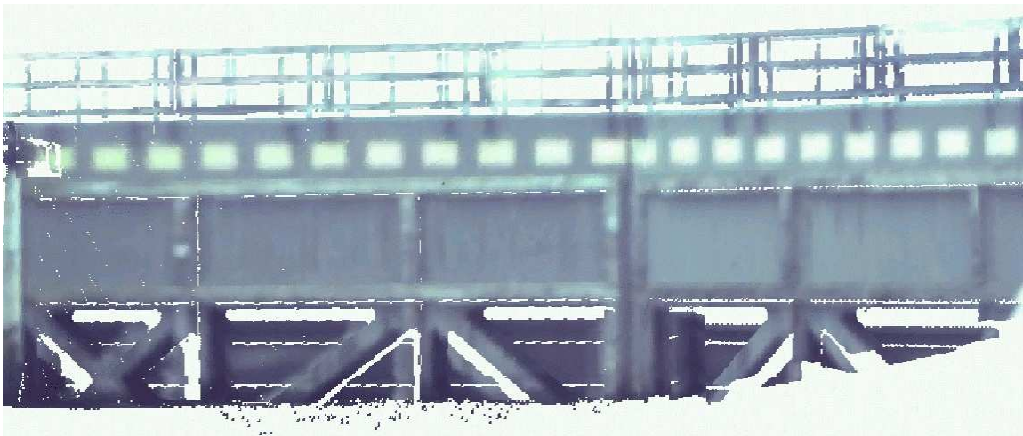
Figure 1: Points from the first scan, representing the lock, colored by the RGB values as photographed by the scanner's internal camera. At the bottom some scan shadows are visible.
