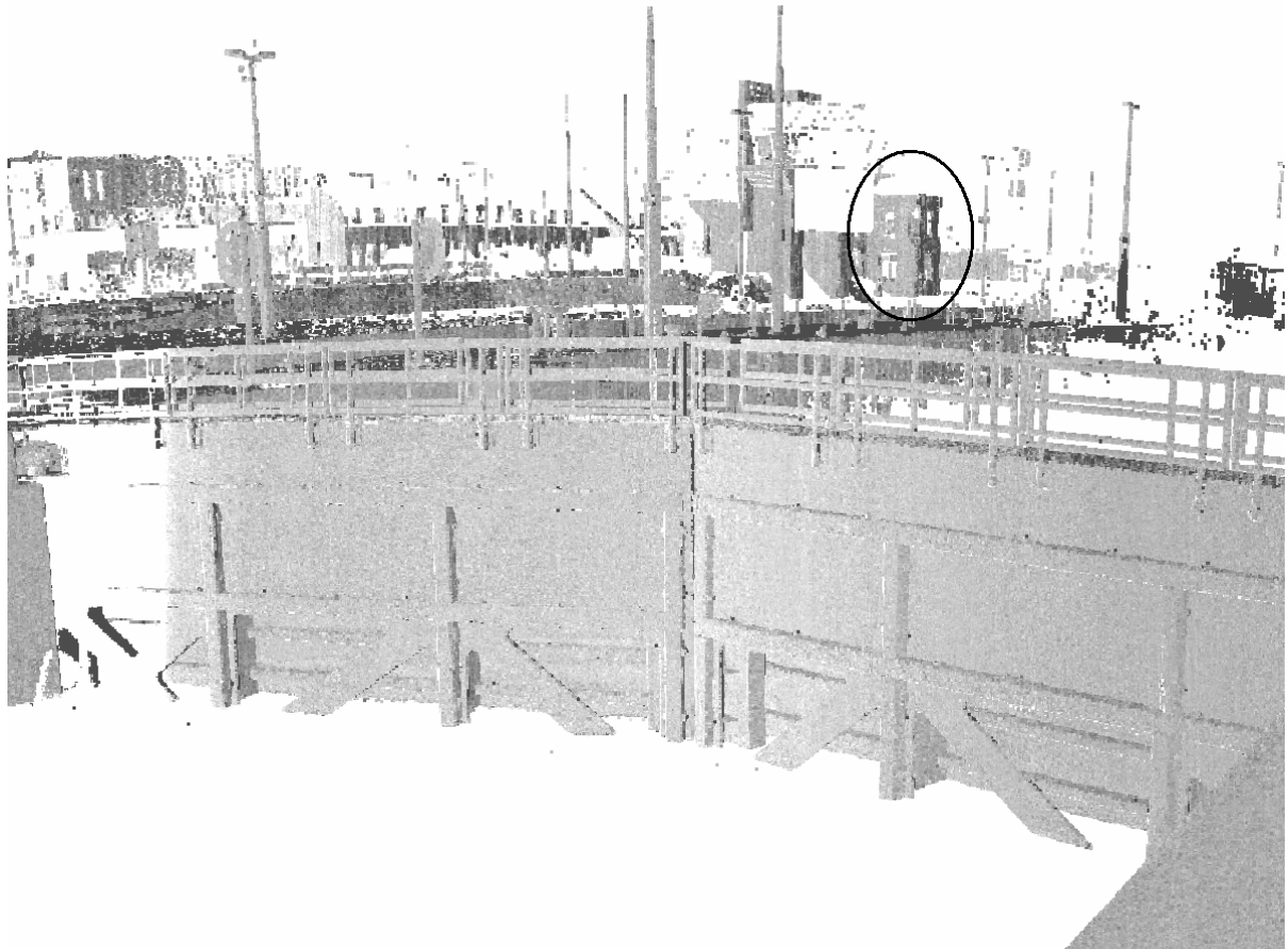
Figure 2: Signed differences in range between Scan 2 and Scan 1 using a direct comparison. Light grey tones indicate a positive difference exceeding 3cm (i.e. the points are further away from the scanner in Scan 2 than in Scan 1), while dark grey is used for negative differences of more than 3cm. Medium grey indicates no movement.
