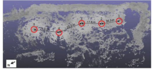
Figure 3. Top view of the scans of the East face after the blast. The scan positions are indicated by red circles.
